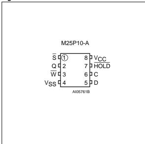
Note: 1. There is an exposed die paddle on the underside of the MLP8 package. This is pulled, internally, to V<sub>SS</sub>, and must not be allowed to be connected to any other voltage or signal line on the PCB.
